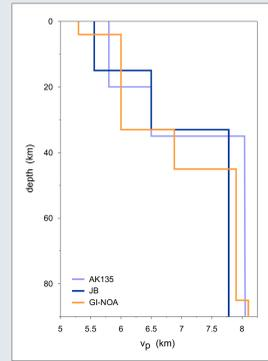
**Figure 1.** Crust and upper mantle representation according to the velocity models used in this study for P-type velocity.
