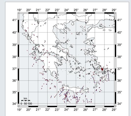
**Figure 9.** Epicentre dislocation vectors for the ISC - AK135 (blue) and the ISC - JB (red) solutions (arrow head), in respect to corresponding EMSC solutions, for the 259 common events between the two bulletins used in this study.
