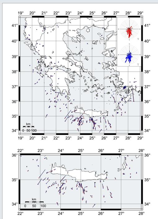
**Figure 6.** Epicentre dislocation vectors for the ISC - AK135 (blue) and the ISC - JB (red) solutions (arrow head), in respect to corresponding ATH solutions, for the 270 events used in this study. Rose-diagrams of the distribution of vector azimuth (top). Same as above, for the broader area of Crete (bottom).
