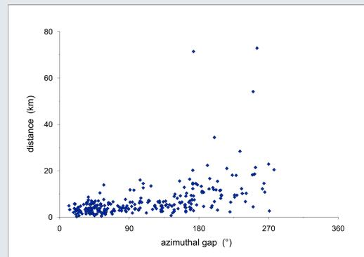
**Figure 4.** Distance between the ISC - JB and ISC - AK135 solutions against ISC azimuthal gap.
