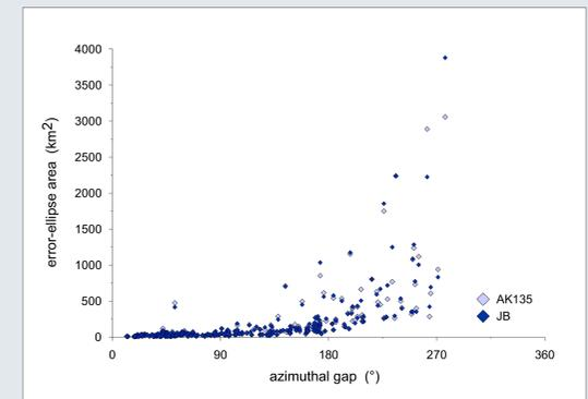
**Figure 5.** Error-ellipse area for the two solutions provided by ISC against azimuthal gap. Since no substantial deviation exist between the two versions, the gap values for AK135 solutions are used.
