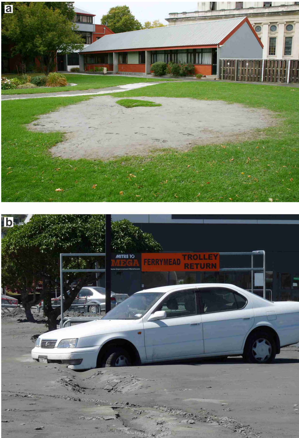
Figure 8.7: (a) Liquefaction area behind the Catholic Basilica, Christchurch, photographer Margaret Low, copyright GNS Science, VML ID 6141. (b) Car trapped by liquefaction, photographer Andrew King, copyright GNS Science, VML ID 101933.
